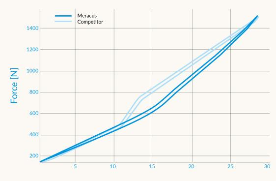
Mechanical tests show that metal fasteners can result in a stiffer product at the forefoot area. With our composite rivet technology, Meracus® presents a deflection that is evenly distributed throughout the forefoot.
